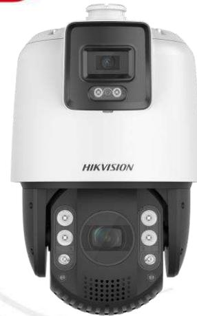
Hikvision DS-2SE7C144IW-AE(32x/4)(S5) 4 MP 32 × IR Network Speed Dome adopts 1/2.8" progressive scan CMOS chip. With the 32 × optical zoom lens, the camera offers more details over expansive areas. This series of cameras can be widely used for wide ranges of high-definition, such as rivers, roads, railways, airports, squares, parks, scenic spots, and venues, etc.
